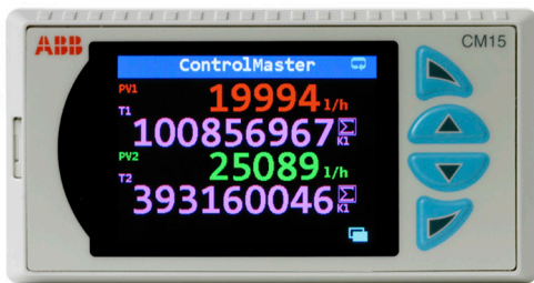
Figure 3 Dual PV and totalization display
