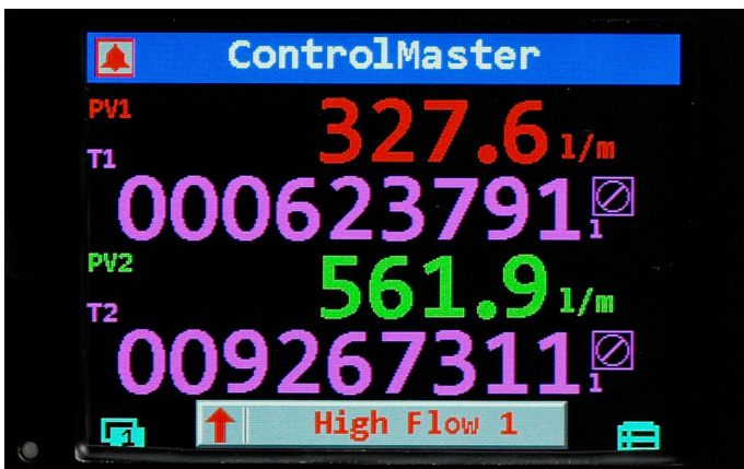
Fig. 3: Dual PV and totalization display
