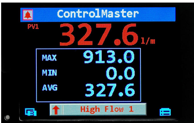
Fig. 2: Single PV indication template display
