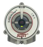
The FV-40 Triple IR detects fuel and gas fires at long distances with the highest immunity to false alarms—it can detect a 1 ft.² (0.1 m²) gasoline pan fire at 215 ft. (65 m) in less than five seconds. The housing is the most durable and weather-resistant design available. It also features a heated window to eliminate condensation and icing, HART capabilities for digital communications, lower power requirements, and a compact, lighter design.
